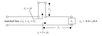
9. Use a single series stub tuner to match the above line to its normalized load. Use a shorted stub and find its distance from the load,  $\ell_1$ , and its length  $\ell_2$ .
