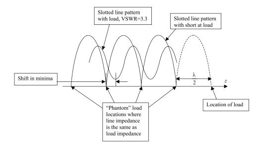
5. An air-filled 50 $\Omega$  coaxial line has a loaded VSWR of 3.3 at a frequency of 3GHz. Replacing the load with a short causes the voltage minimum to move 1.0 cm towards the generator. What is the normalized load impedance?
