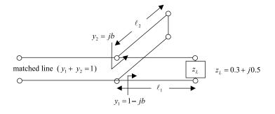
10. Use a single parallel stub tuner to match the above line to its normalized load. Use a shorted stub and find its distance from the load,  $\ell_1$ , and its length  $\ell_2$ .
