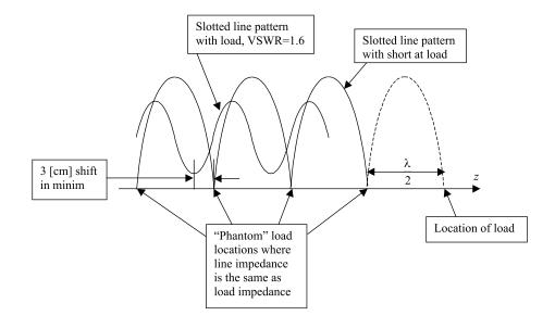
6. A slotted line measurement on an air-filled TEM line yields a VSWR of 1.6 at a frequency of 1 GHz. When the load is replaced by a short, the voltage minimum moves 3 cm towards the load. Find the normalized load impedance.
