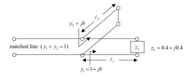
8. Use a single parallel stub tuner to match the above line to its load. Use a shorted stub and find its distance from the load,  $\ell_1$ , and its length  $\ell_2$ .
