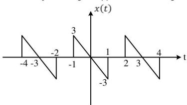
A signal g(t) is defined by  $g(t) = x\left(\frac{t-1}{2}\right)$ . The average power of g(t) is
