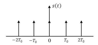
The given impulse train s(t) with strength of each impulse as 1 is aperiodic function with period  $T_0$
