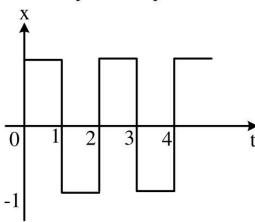
The ratio of the power in the 7<sup>th</sup> harmonic to the power in the 5<sup>th</sup> harmonic for this waveform is closest in value to -----
